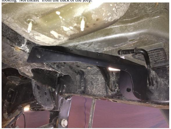
I did not install the rock stars, and instead opted for the high-clearance weld on kit. So I cannot comment on installing those and connecting the bottom of the coil overs, but it looks fairly straightforward in the instructions. You do have to cut some things to install the rear coil overs: The factory track bar mount on the axle and the bottom part of the lower control arm (for the rock stars).
